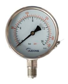
working environment and can also decrease the ripple effect from the medium. Pressure Gauges are constructed with a bourdon tube sensing element. When the sensing element is subjected to pressure, it flexes and the resulting motion is transmitted as a measurement through a mechanical movement to the dial face pointer.
